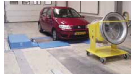
Car on VLT 148950 with cooling fan
